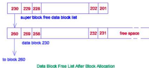
Fig. 3.16: Free list after allocating some data blocks
